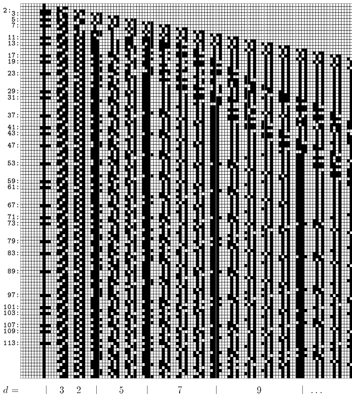
Figure 3. Real-time generation of the primes by a 2-state 1D CA with r \leq 10 .
